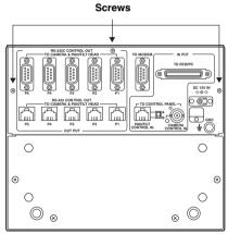
4. Use the three screws to firmly secure the blank panel where the rear panel was removed.
